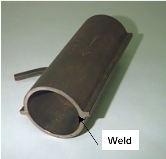
2.5" x .155" steel fin boiler tube
